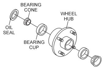
Figure 29. Wheel Hub and Bearings
